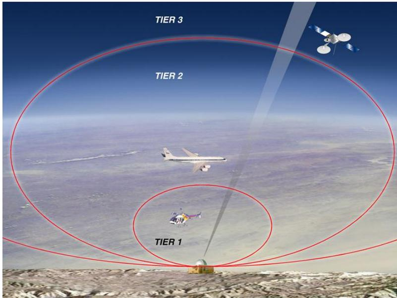
**Figure 61: OCTL's Three-tiered safety system**
