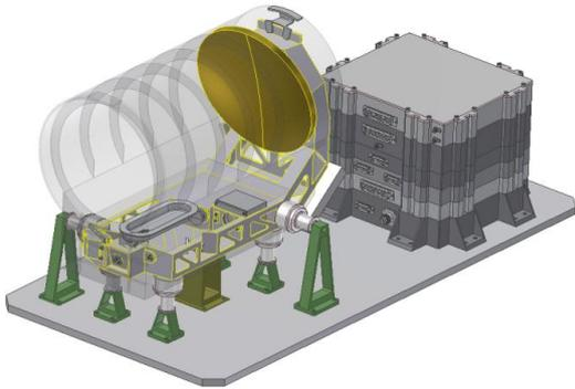
**Figure 46: 22 cm DOT Flight Terminal with Vibration Isolation and Opto-Electronics Box**
