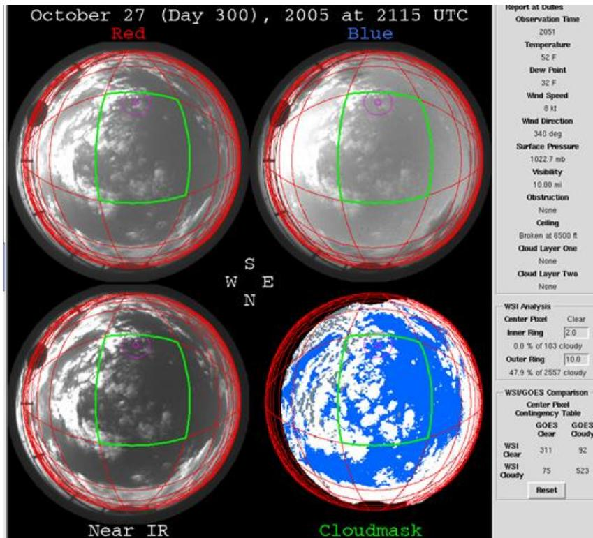
**Figure 5: Example of a Whole Sky Imager (WSI) that could be used to support link handover decisions for a free space optical communications network**
