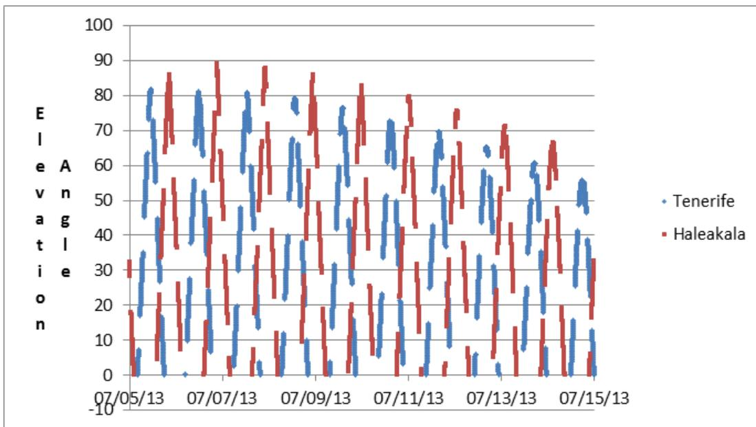
**Figure 30: Geometric Access from LLST to hypothetical ground terminals at Haleakala and Tenerife (from July 5 – 15, 2013).**
