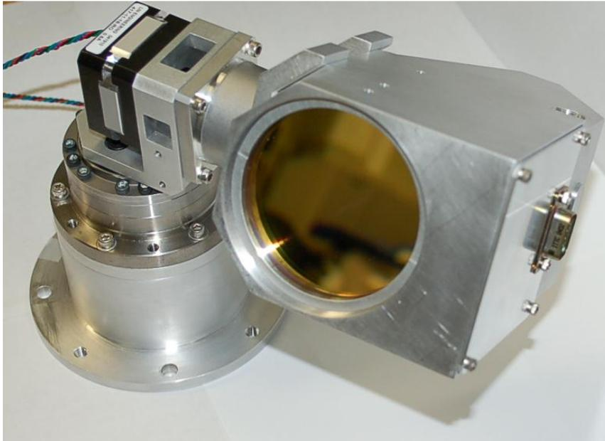
**Figure 20: The optical-head prototype for laboratory and in-the-field (communications from an airplane) testing.**
