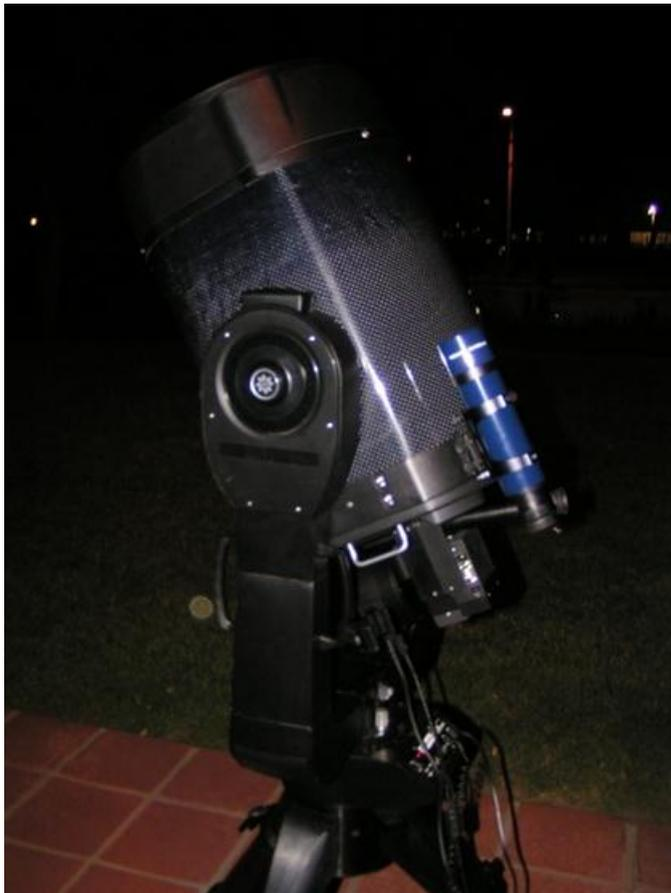
**Figure 9: DIMM for measurements of nighttime turbulence.**
