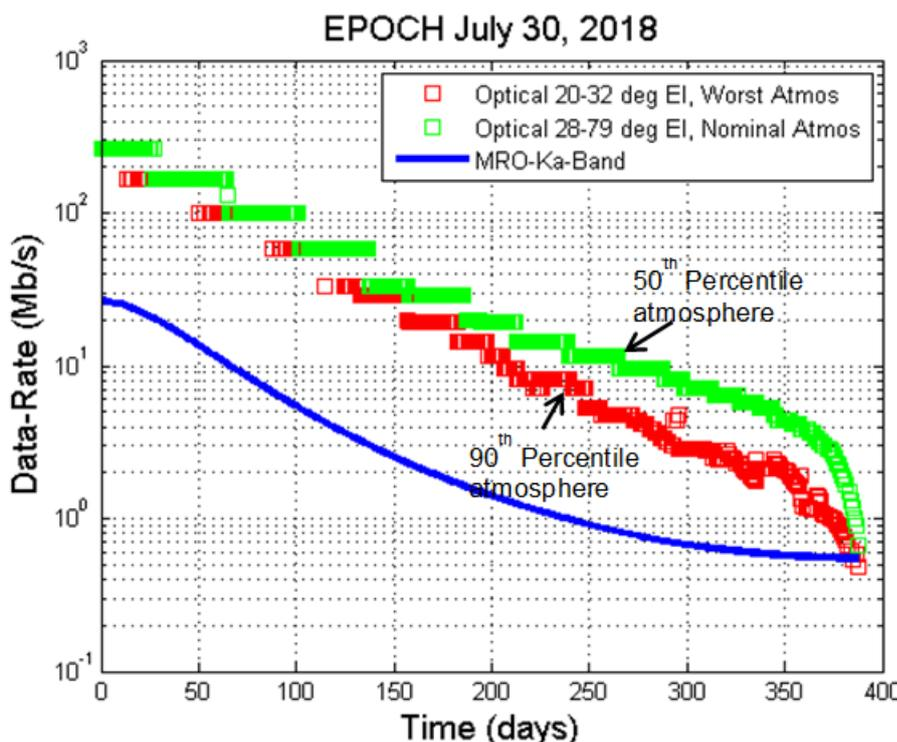
**Figure 42: Data rate vs. distance at GDSCC**
