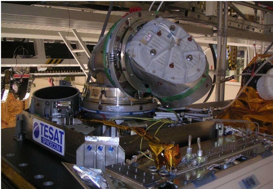
**Figure 55: Laser communication terminal with hemispherical coarse pointing periscope actuated**
