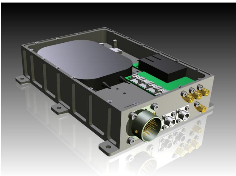
**Figure 17: Laser Source using an optical amplifier**
