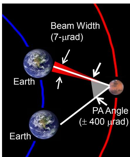
**Figure 4: Point Ahead Angle Example**
