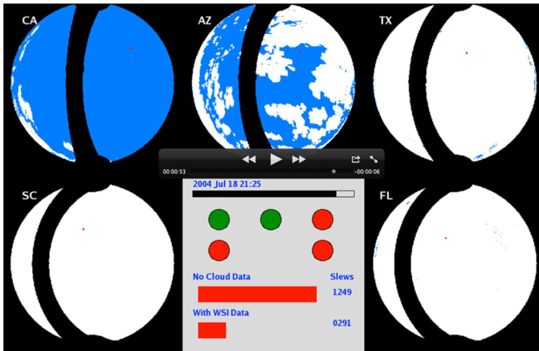
**Figure 1: Lasercom Simulator output showing the benefit of local cloud instrumentation on minimizing link handovers.**
