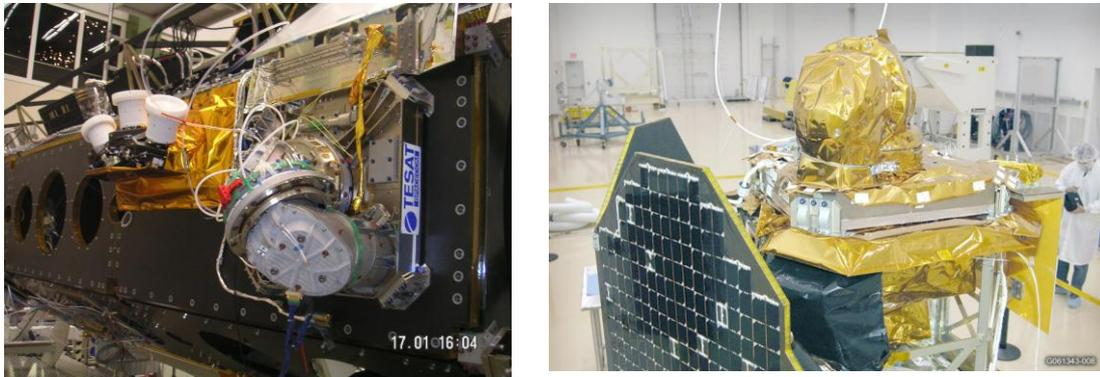
**Figure 18: Tesat laser communication terminals embarked on the TerraSAR-X (left) and the NFIRE (right) satellites**
