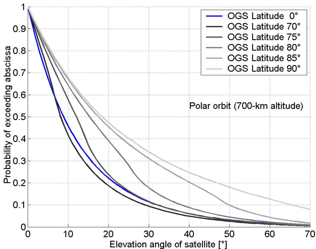
**Figure 14: Probability distribution of the satellite elevation (assuming the satellite is above the OGS horizon).**
