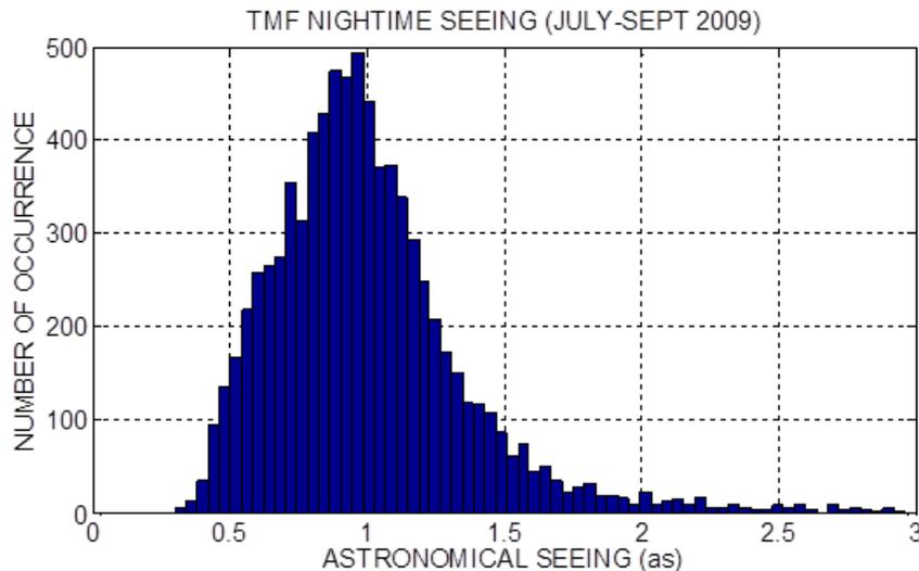
**Figure 10: Histogram of astronomical seeing at Table Mountain Facility, CA. The data is from measurements by a DIMM during the period July-Sept, 2009.**
