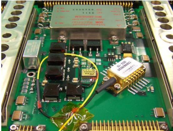
**Figure 16: Space-qualified directly modulated laser diode**
