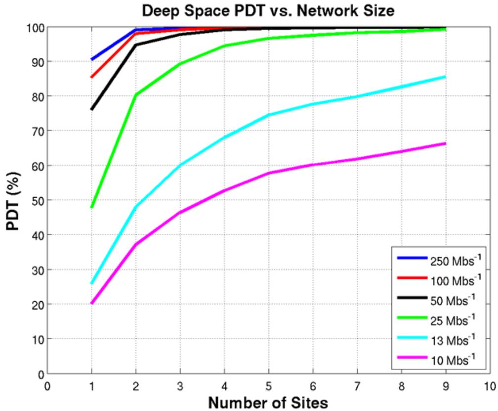
**Figure 50: Overall Percent Data Transferred (PDT) for the Deep Space scenario for 1-9 site networks of ground stations for six different data rates.**
