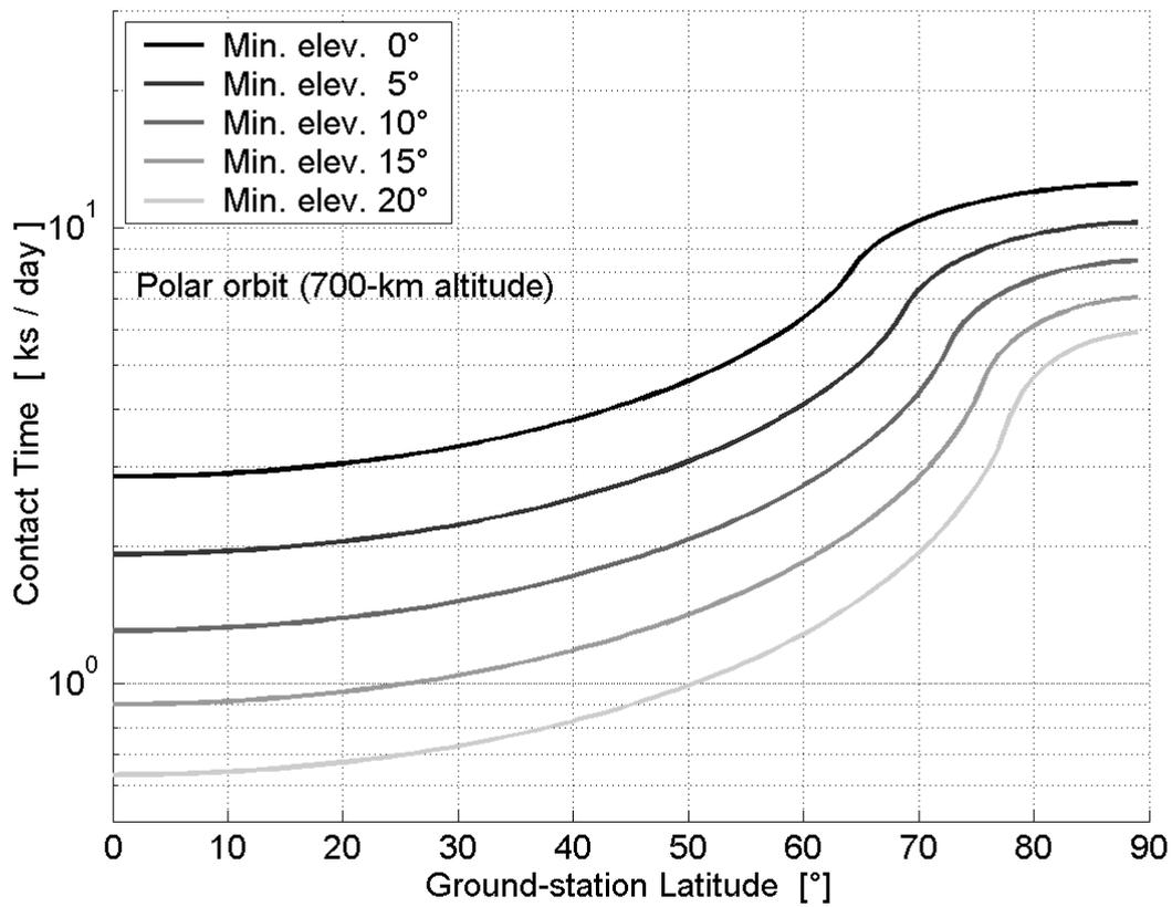
**Figure 13: Orbit-limited contact time per day as a function of the ground station latitude for a polar-orbit satellite.**
