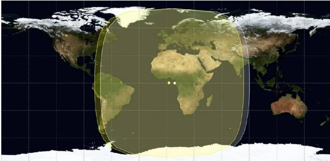
**Figure 54: Planned orbital locations and Earth coverage of the first two EDRS satellites EDRS-A (9° East) and EDRS-C (3° East, TBC)**
