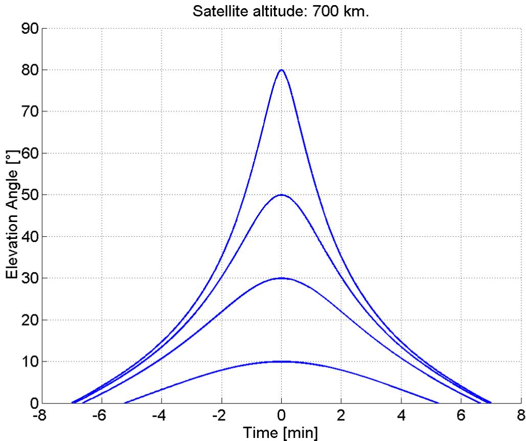
**Figure 12: Elevation angle versus time for satellite overflights with various maximum elevations**
