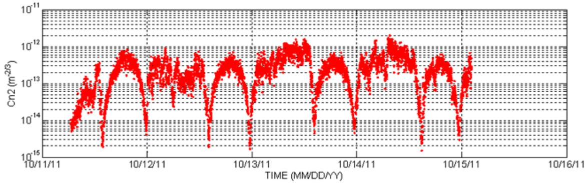
**Figure 11: Measurements of the ground layer structure coefficient of the refractive index at Goldstone. (Time is in UTC).**
