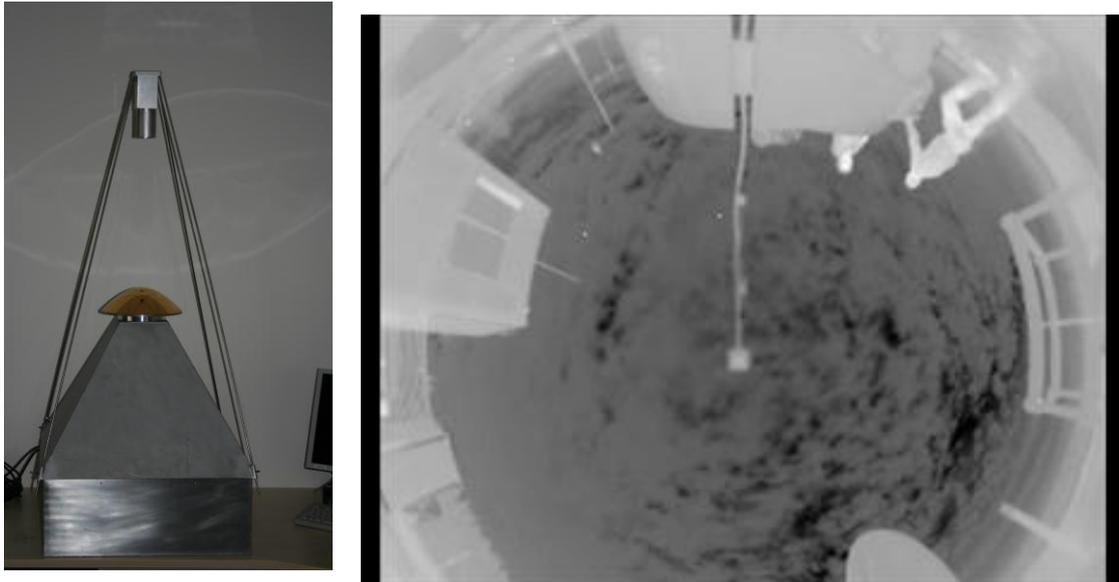
**Figure 6: Set up of the CloudCam (left) and example image of cloud situation over the optical ground station Oberpfaffenhofen (right).**
