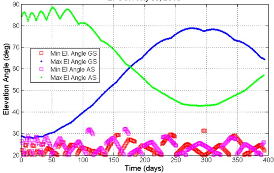
**Figure 39: Elevation angles of a Mars-orbiting spacecraft relative to GDSCC and Alice Springs**
