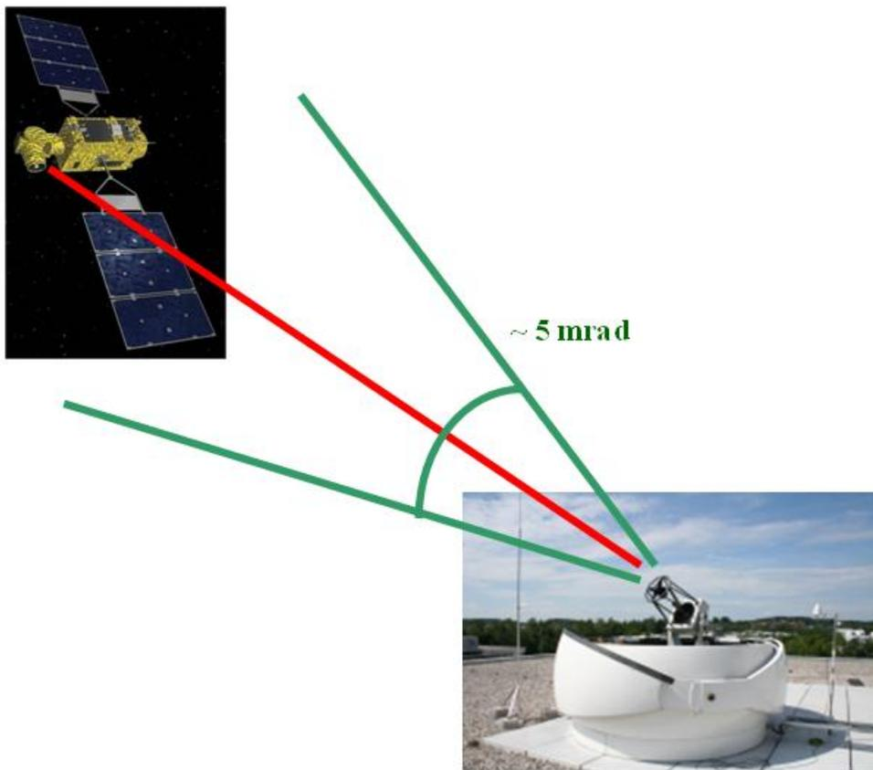
**Figure 15: Illustration of a large beacon beam (divergence  $\sim 5$  mrad) emitted by an OGS and a narrow communication beam emitted by the satellite.**
