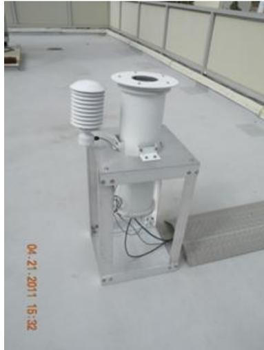
**Figure 8: NASA-JPL cloud camera. The window visible in top of the weatherproof enclosure is made of hard coated germanium.**
