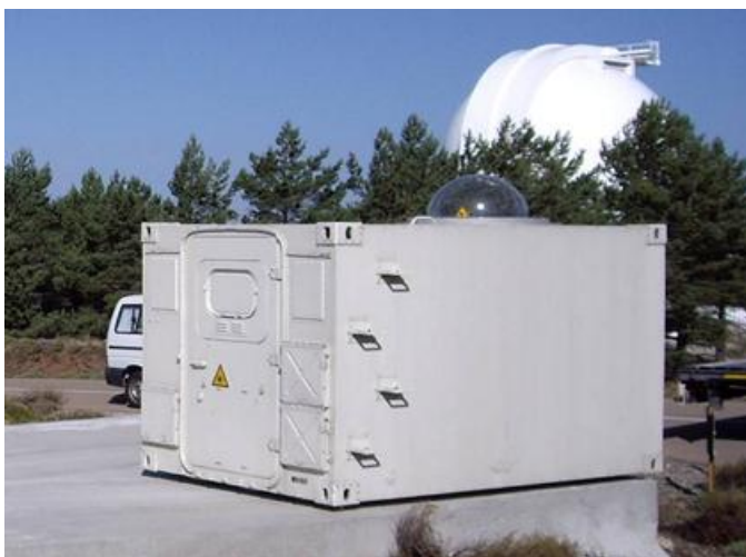
Figure 70: The transportable adaptive optical ground station currently developed by Tesat is fitted into a standardized shipping container.
