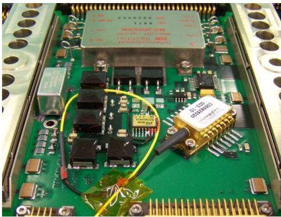
Figure 15: Space-qualified directly modulated laser diode.
