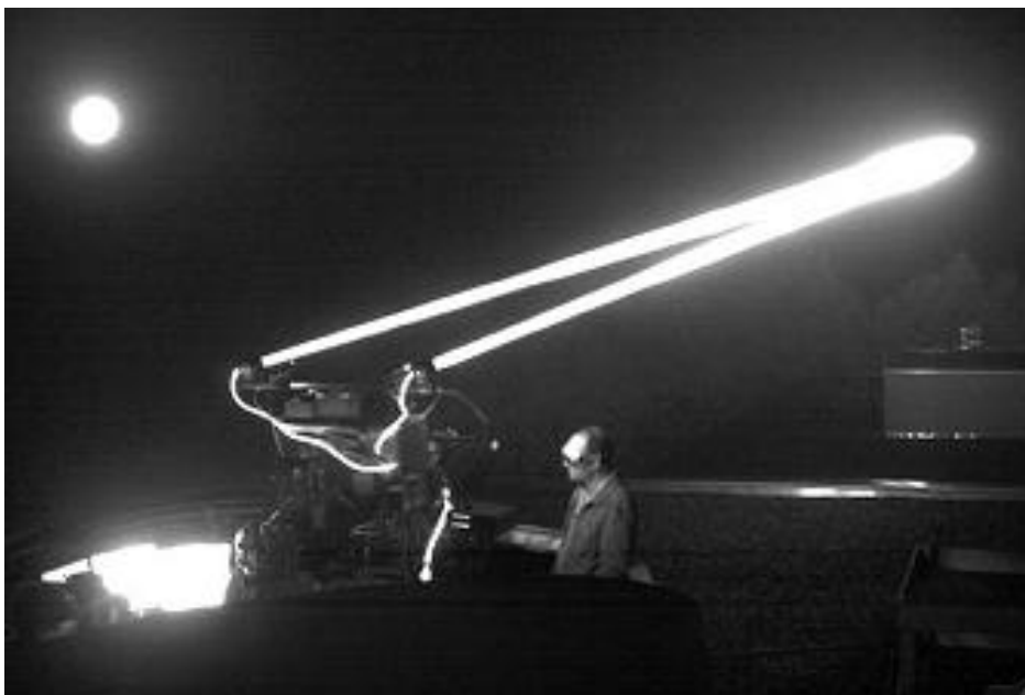
Figure 23: DLR's OGS at Oberpfaffenhofen during a laser link with the OICETS satellite at nighttime (2009). The two infrared uplink beacons can be seen.
